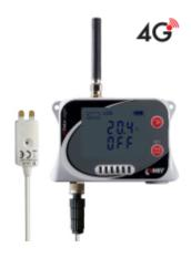
The U3832G datalogger is used to measure temperature, relative humidity and dew point temperature using internal sensors, plus an attached LD-81 flood detector to indicate water flooding. In case of exceeded set limits, SMS and JSON messages can be sent via 4G data connection. Measured values can be sent to the internet storage COMET Cloud, which is a complete monitoring, alarm and analysis system.
